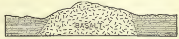
FIG. 21.—Pilot Knob, Texas, a volcanic plug. (After Hill, U. S. Geological Survey.)
